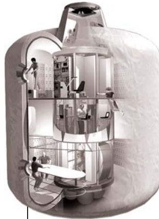
NASA TransHab 1990s "Transit Habitat" for Mars Rigid Core with Cylindrical Inflatable
